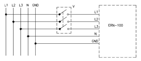
Note: An additional switch "V" is recommended to use in case, if the lead-in cable is fixly connected to the line distribution. If the moving terminal is used for the installation, this switch will be not necessary.
