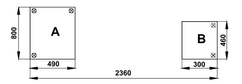
Surfaces A and B must be balanced horizontal in one surface. The winding machine is moved by lifting at 3 pendant eyes. At the winding of heavy coils there is recommended to fix the base frame with screws M 12 directly to flooring surface in marked points.
