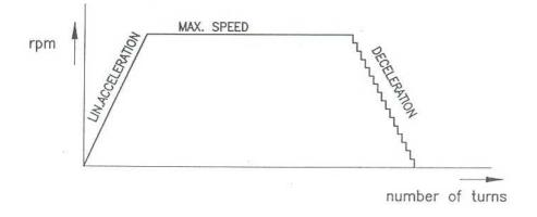
Deceleration is microprocessor-controlled, which ensures an accurate stopping and positioning of the spindle at minimum winding time.
